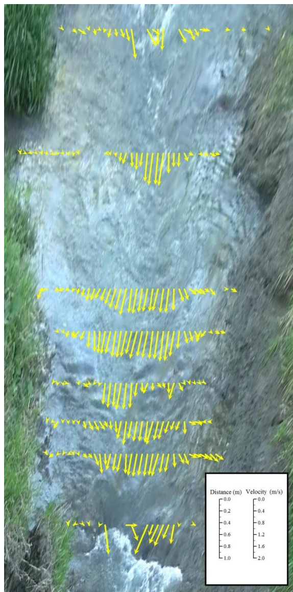
Figure 5.5: Surface water velocity distributions created from LPIV data collected on September 27, 2011 site visit.
