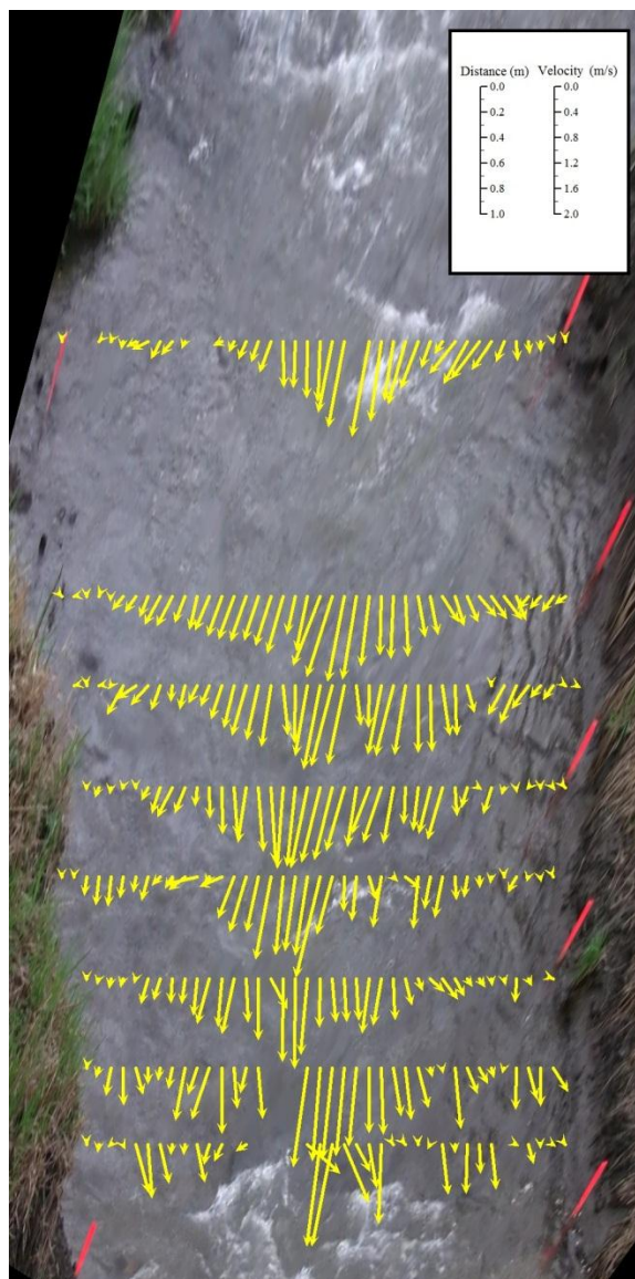
Figure 5.6: Surface water velocity distributions created from LPIV data collected on March 21, 2011 site visit.
