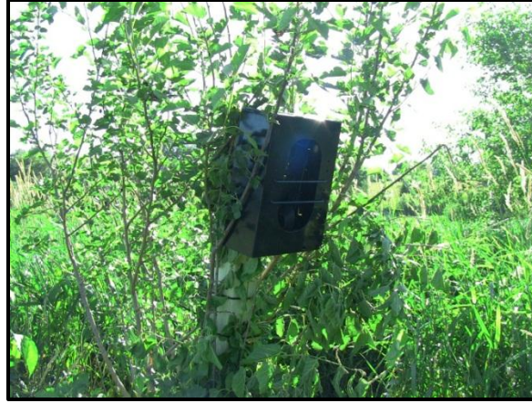
Figure 3.4: Time lapse camera installation at site
